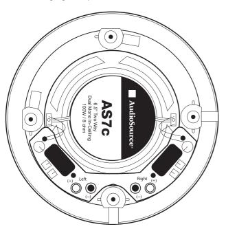
The AS7c uses a dual voice coil woofer and dual tweeters. The speaker has separate terminals to allow each channel of a stereo amplifier to be connected to the one speaker.
